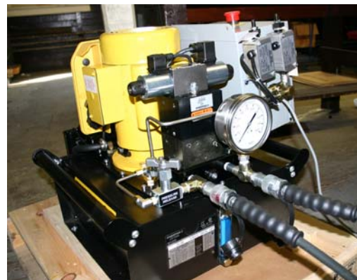
HYX-508 Hydraulic Tubing Crimper Above—Jaw Crimping Tubing Right—Hydraulic Unit Powering Tubing Crimper
